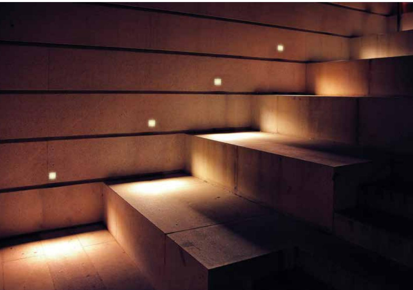
The Wall Recessed range consists on a set of luminaires suitable for halls, stairs or other lighting purposes near to the mopboard. These products, which may have 1W or 4W, have a high IP rating, a CRI higher than 85 and asymmetric beam angles, technical features needed in this type of light fitting.
