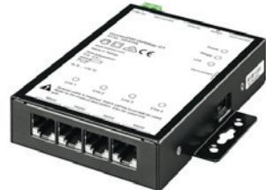
FULL Smart is a more complete system that allows you to program and control the lighting fixtures remotely, from the other side of the world, thanks to an Internet-based Gateway, designed for buildings with a more advanced lighting system. This system allows to detect failures in damaged fixtures in the building. Some diagnostic and maintenance operations can be performed through the FULL Smart system.
