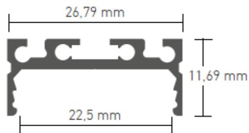
NP04 ALUMINIUM PROFILEPRODUCT TABLE AND TECHNICAL SPECIFICATIONS - NP04 aluminium profile - 2000mm x 26,79mm x 11,69mm - for LED Strip up to 24mm
