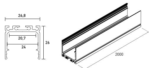
**NP06 ALUMINIUM PROFILE****PRODUCT TABLE AND TECHNICAL SPECIFICATIONS - NP06 aluminium profile - 2000mm x 26,8mm x 26,00mm - for LED Strip up to 24mm**
